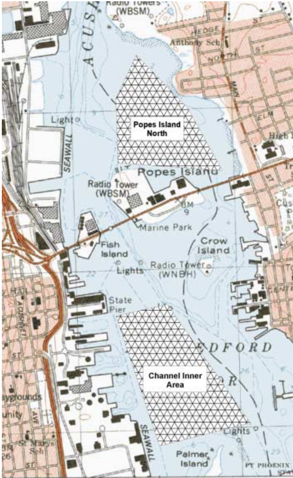
Figure 1-1. Proposed preferred alternatives CI and PIN CAD cell areas in New Bedford/Fairhaven Harbor
